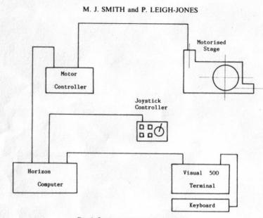
FIG. 1. System components and connections.
